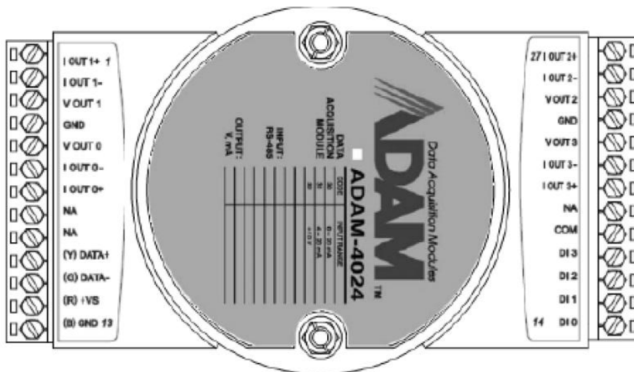
Figure 3: Connection pins of the ADAM-4024 module
